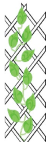
Erect a trellis to reduce sun exposure
